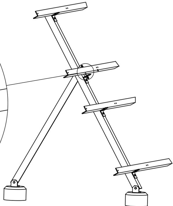
Install WEEB-9.5 NL to bond support frame and panel mounting frame
