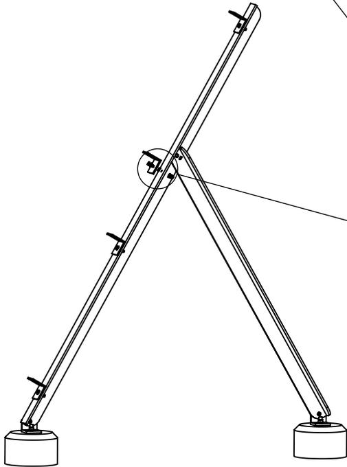
Install WEEB-9.5 NL between angle bracket and mounting frame.
