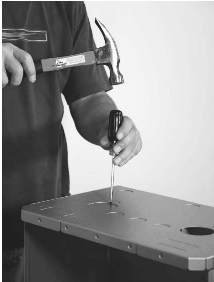
Figure 6: Removing chassis side knockouts
